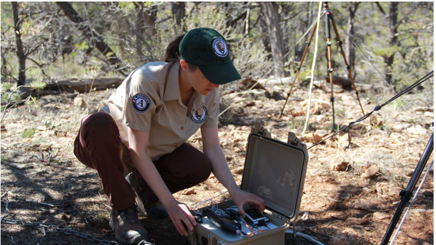
GIP Hannah Chambless preparing sound level meters as part of an acoustic monitoring project in Grand Canyon National Park, Arizona. (NPS photo)
